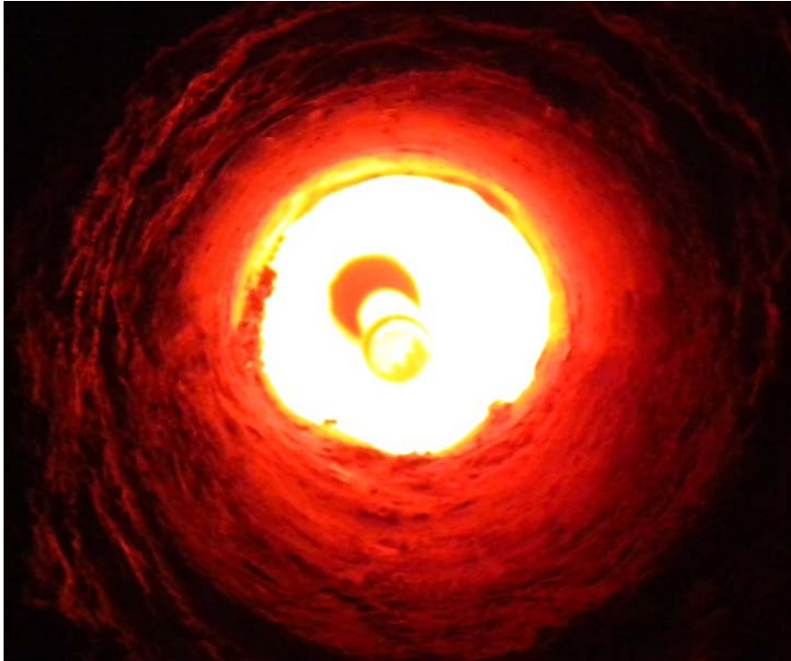
Superheat corrosion probe (347h)
